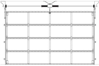
Max door height: 3.5m, Max door weight: 240kg, Max door area: 18.5m<sup>2</sup>
