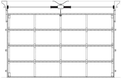
Max door height: 3.5m, Max door weight: 240kg, Max door area: 18.5m<sup>2</sup>
